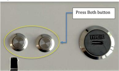
Locate the two small metal buttons on the front side of the controller
